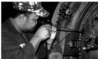
Borescope inspection For Preventative Maintenance.
